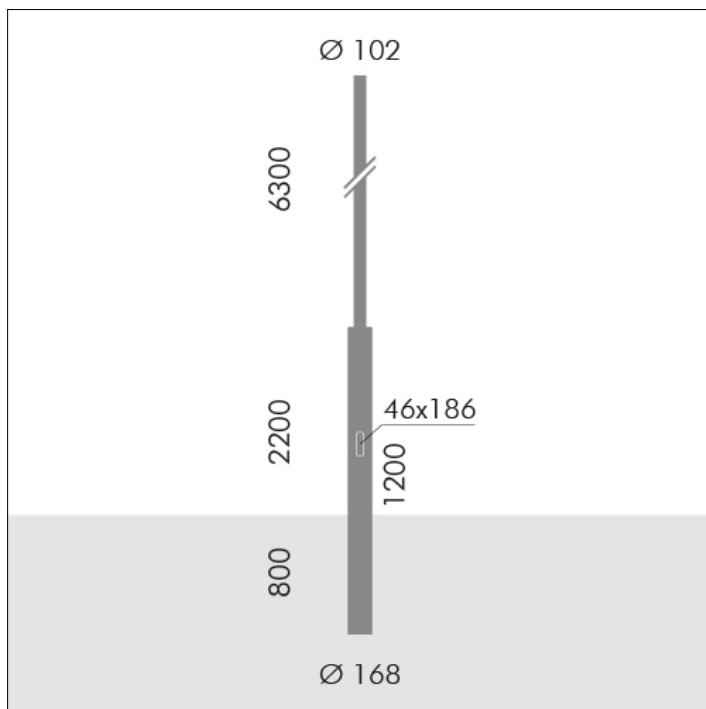
**S.2817****CYLINDRICAL SHAPED POLE H 8,5m Ø 168mm -
