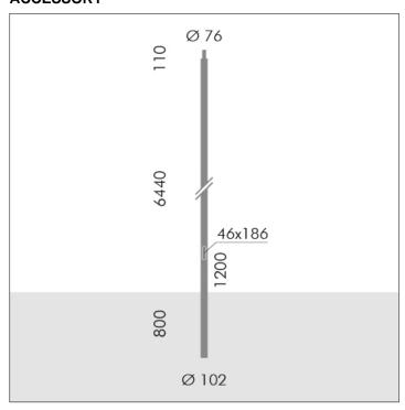
S.2818 H 6,44m Ø102mm CYLINDRICAL POLE TO BE BURIED with Ø76mm SPIGOT
