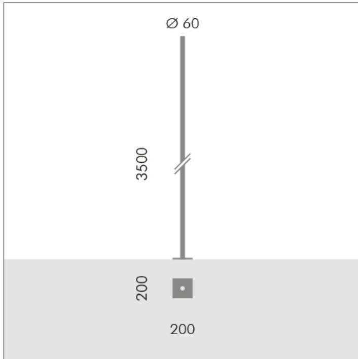
**S.2843****H 3,5m Ø60mm CYLINDRICAL POLE WITH BASE**
