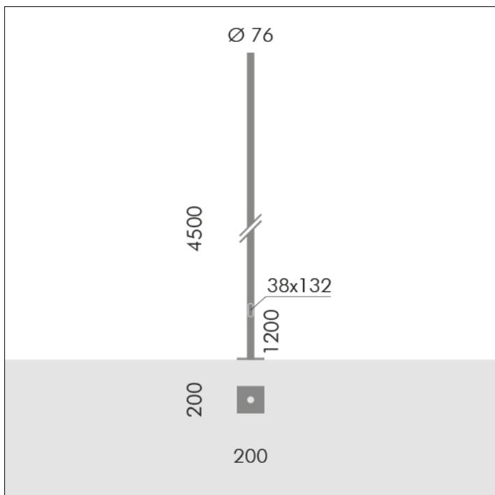
**S.2845****ZYLINDRISCHER MAST H 4,5m Ø76mm MIT
