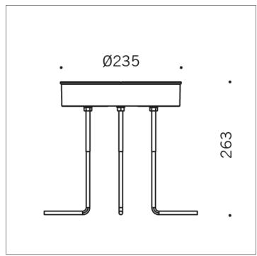
S.5690 ANCHOR FLANGE TO BE CEMENTED TO THE GROUND
